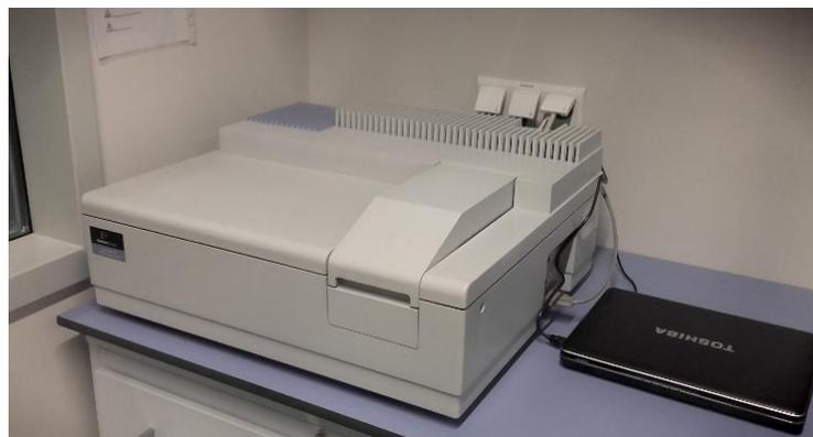
Slika 9. UV VIS spektrofotometar Perkin Elmer Lambda 25, double beam.
