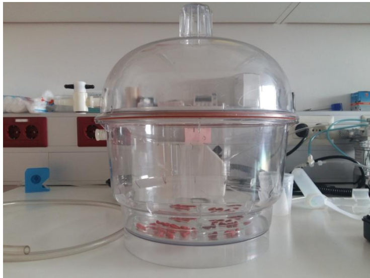
Slika 9. Vakumska posuda (Thermo Scientific Nalgene 5311-0250 Vacuum Desiccator).
