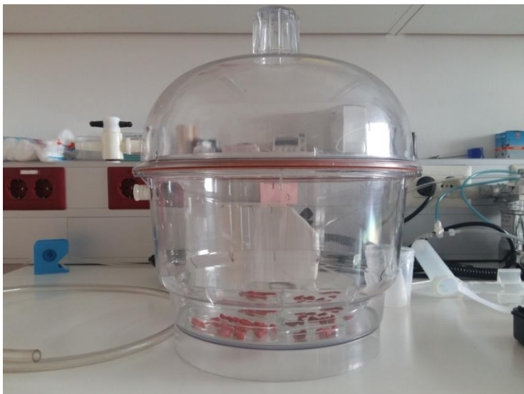
Slika 9. Vakumska posuda (Thermo Scientific Nalgene 5311-0250 Vacuum Desiccator).
