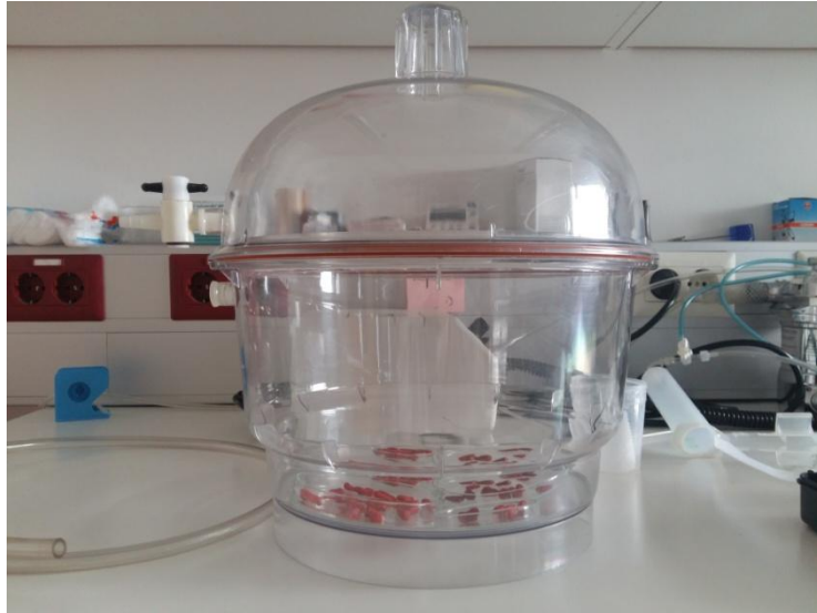
Slika 9. Vakumska posuda (Thermo Scientific Nalgene 5311-0250 Vacuum Desiccator).
