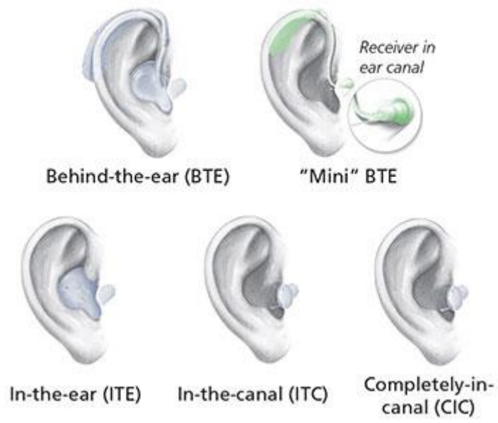
Figure 7. The different styles of hearing aids (31).
