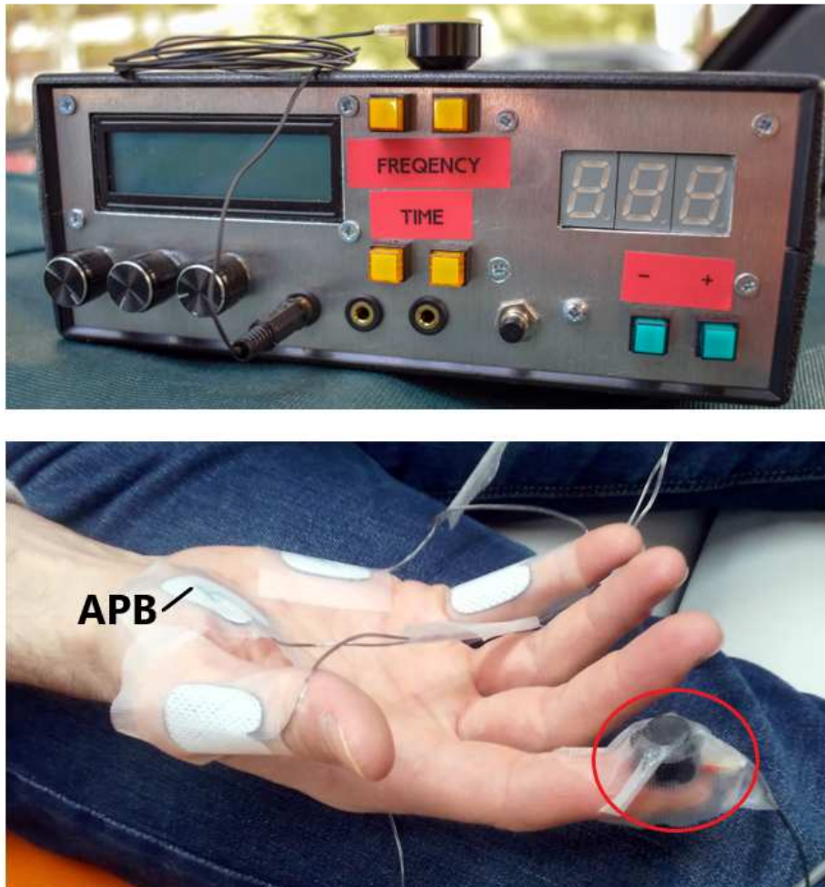
Figure 2. Upper: vibration controller; Lower: Vibrotactile stimulator (circled) and the EMG electrodes in the configuration used. Source: Laboratory for Human and Experimental Neurophysiology, School of Medicine, Split.
