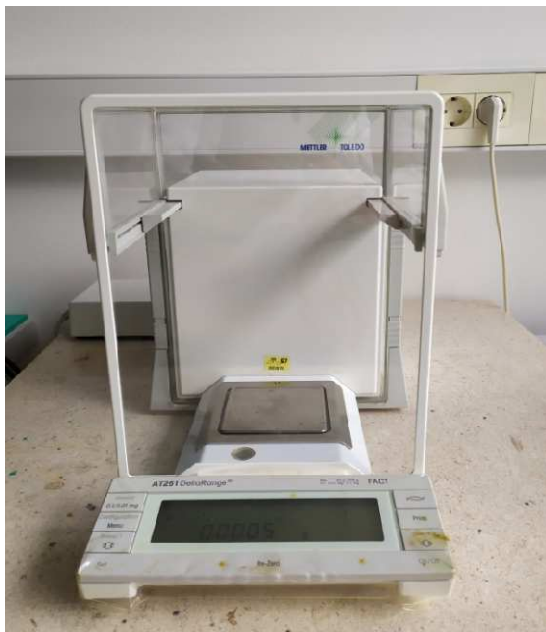
Slika 1. Vaga (AT261 DigitalRange, Mettler Toledo)
