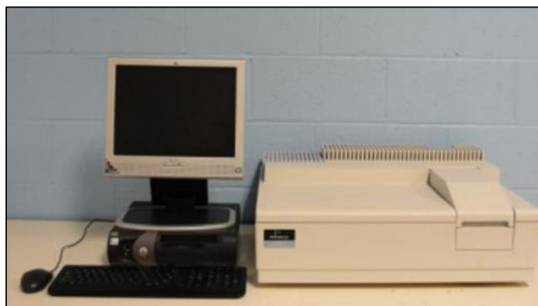
Slika 2. UV-Vis spektrofotometar Perkin Elmer Lambda 25, double beam
