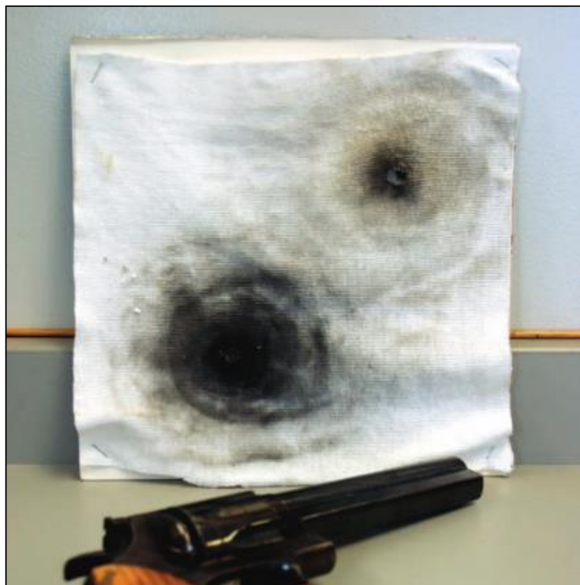
Figure 4. Comparison of shooting distance as seen in GSR. The closer the shooter is to the victim, the darker the GSR. Source: (39).
