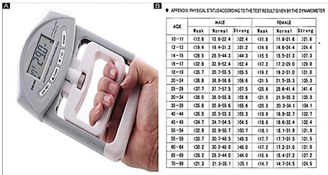
Figure 2. (A) Handgrip dynamometer; (B) Reference values for handgrip strength. Source: (16).
