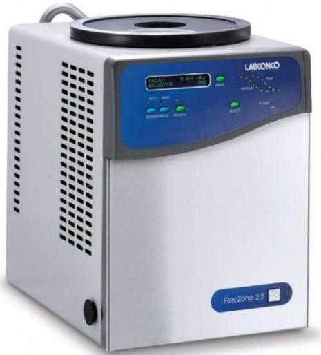
**Slika 7.** FreeZone 2.5 Liter Benchtop Freeze Dry System uređaj (46).
