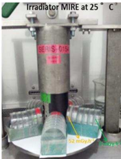
Figure 14. Used 137 Cs source for IR.
