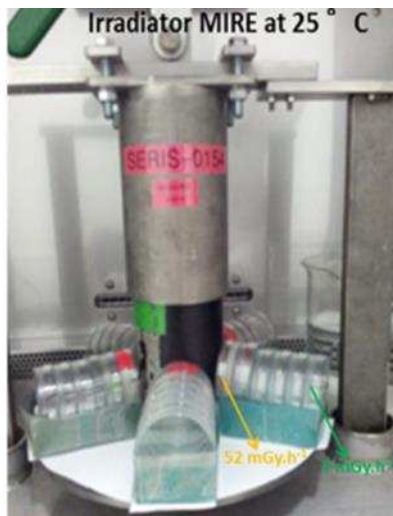
Figure 14. Used 137 Cs source for IR.
