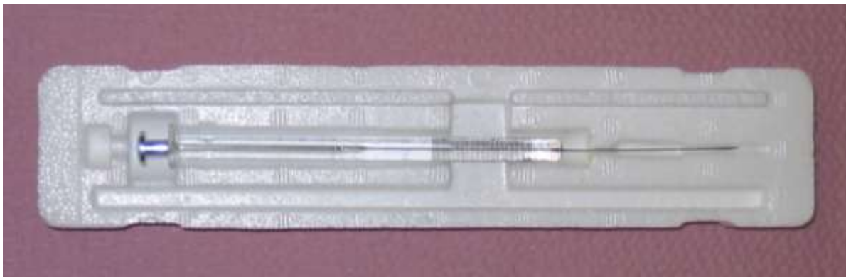
Slika 6. Hamiltonova štrcaljka, (Dynatech Precision Sampling Corp., Baton Rouge, SAD)
