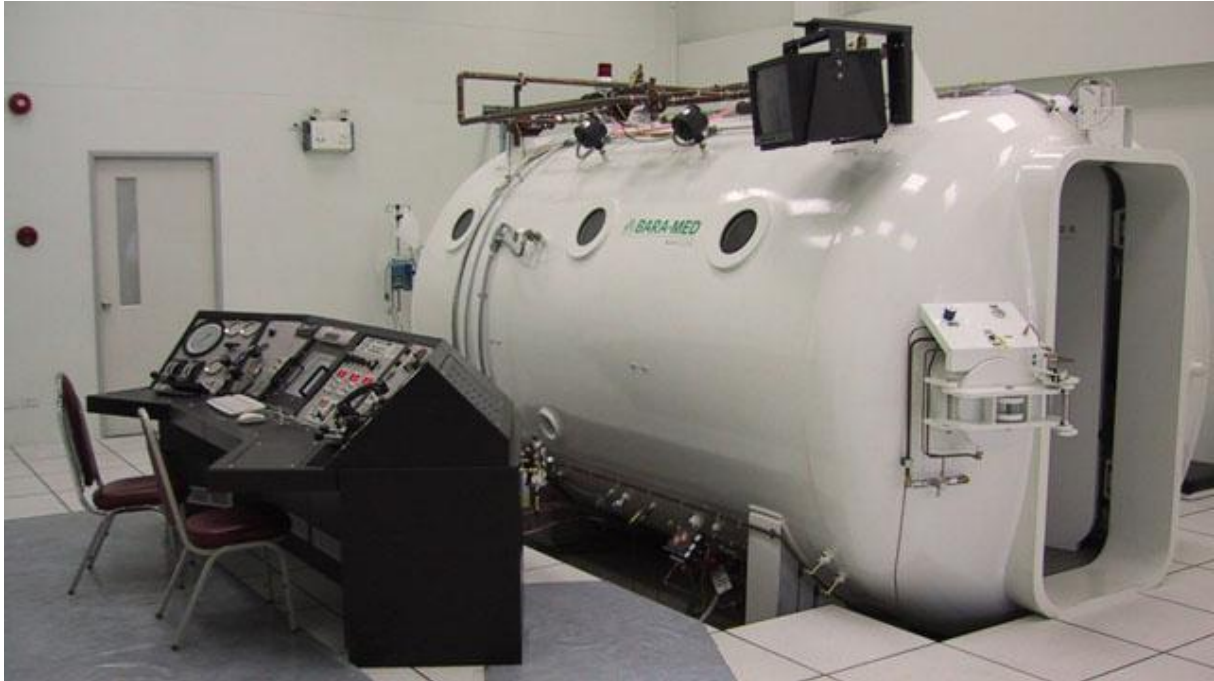
Slika 7. Hiperbarična komora (preuzeto sa: http://www.etcaerospacesolutions.com/wp-content/media/product/images/chamber-main.jpg )
