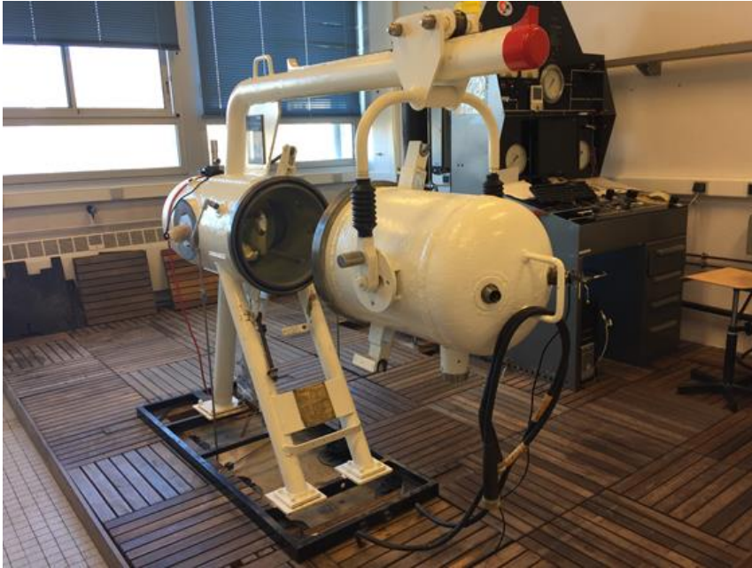
Figure 12. Opened 130-l steel decompression chamber.
